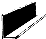
Unequal-leg steel angle L 6 × 4 × 3/8"
